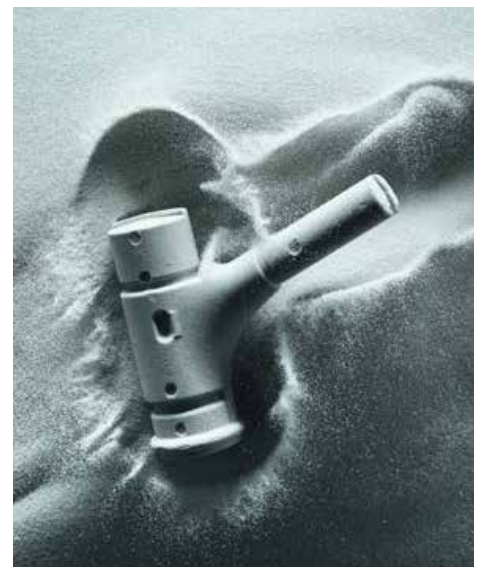
Using low pressure die casting, the brass is melted and then poured into sand moulds
