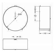
Jumbo roll holder for wall mounting, stainless steel, surface satin finished, material thickness 0.8 mm, cylinder lock with Franke standard key, closed round casing with inspection window, paper withdrawal over two tear-off edges, for 1 roll with max.  $\varnothing$  260 mm, incl. stainless steel screws and dowels.
