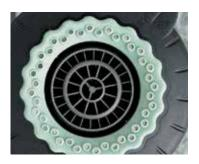
This flexible faceplate reduces the amount of cleaning effort required. When water is flowing, the cone shaped holes expand, dislodging any limescale deposits from the surface of the faceplate. The holes contract automatically when the water flow is switched off.
