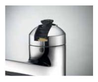
This innovative sealing membrane keeps KWC taps watertight for a long time. It protects the control cartridge from residue left by cleaning agents and dirt. The lever support is reinforced with a metal core and integrated into the membrane, reliably preventing the lever from coming loose.
